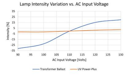
Fig. 2, Startup intensity comparison during line voltage fluctuations encountered at a typical industrial site.
